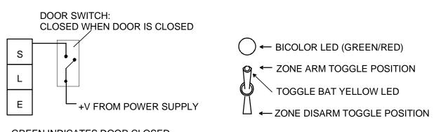
GREEN INDICATES DOOR CLOSED. RED INDICATES VIOLATION (DOOR OPENED WHEN ZONE ARMED). ORANGE INDICATES READY FOR ALARM RESET (DOOR HAS RECLOSED AFTER VIOLATION).
